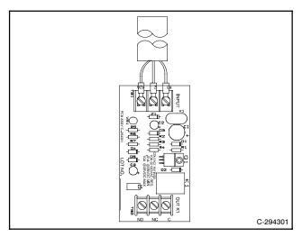
Figure 6-4 Common Failure Relay Kit
